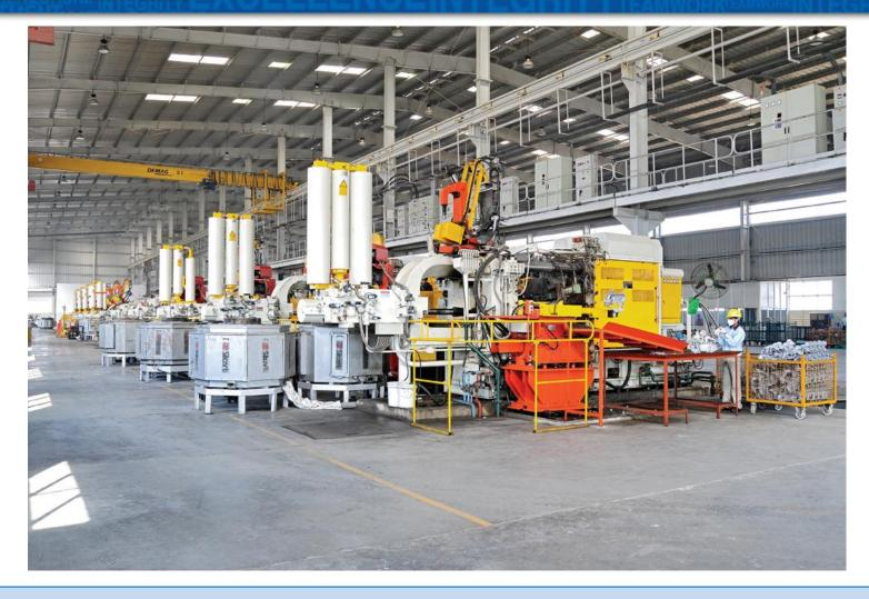
Over 100 High Pressure Die Casting Machines (135 – 2500 Tns Locking Force) Largest High Pressure Die Casting Capacity in India including GDC & LPDC.
